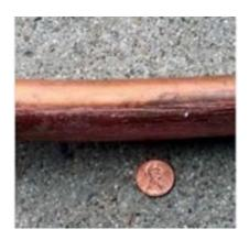
Metal: To find out what kind of metal pipe you have, perform two simple tests: 1) a scratch test with a coin or key; and 2) a magnet test. You will need a key and/or penny and a magnet for these tests.
